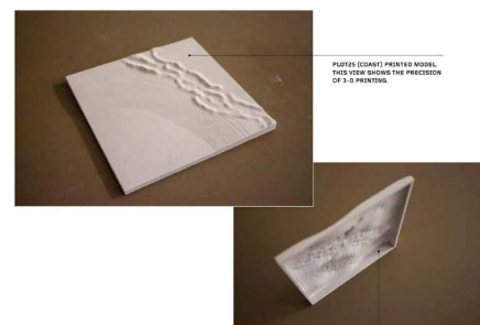
6 FOLLOWED UNDERSIDE OF PLOTS (UPLAND FOREST). THIS TECHNIQUE USES LESS POWDER, WHICH REDUCES COST AND PRINTING TIME
